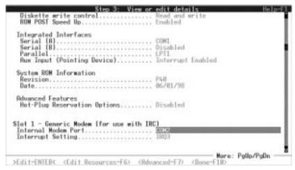
Figure 2-2. Example: Setting the COM and IRQ resources
